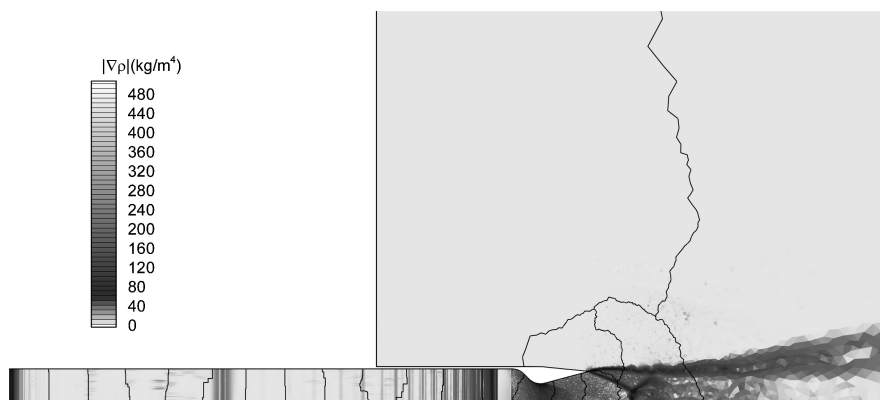
Fig. 14 Density gradient of the flowfield for the baseline condition immediately before the detonation wave reaches the converging portion of the nozzle ( t = 0.07803 corresponds to Fig. 12).
